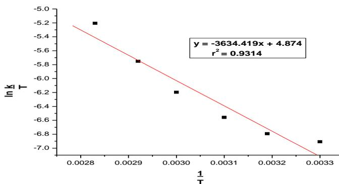
Figure 8. The Eyring curve for yellow oleander oil extraction
