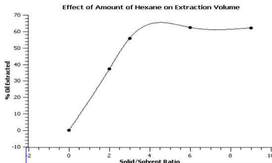
Figure 1. Effect of solid/Solvent ratio
