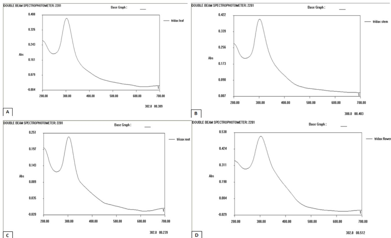
**Fig. 4.** UV-Visible characterization of ZnO nanoparticles; **4A** - UV-Visible absorption spectrum of leaf reaction medium. **4B** - UV-Visible absorption spectrum of stem reaction medium. **4C**- UV-Visible absorption spectrum of root reaction medium. **4D** - UV-Visible absorption spectrum of inflorescence reaction medium.
