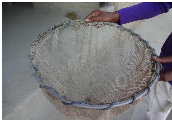
Fig. 1. *Hulcar* a type of hand operated circular scoop net.
